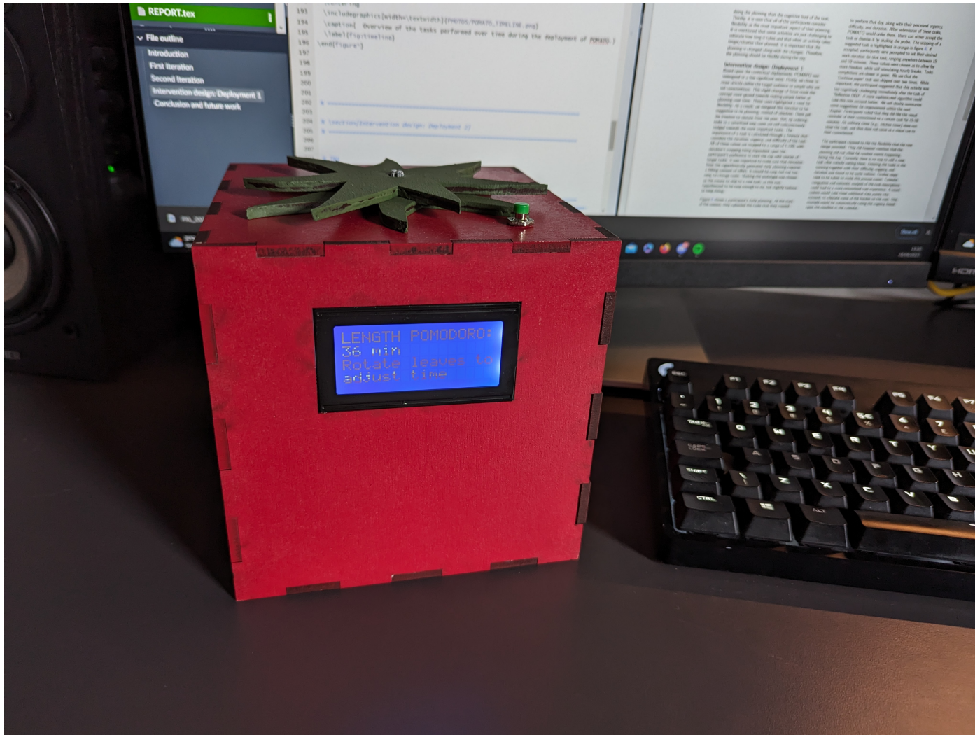
Figure 5: The Intervention Design. The POMATO probe downloads all the daily planning and displays a task for the users to do. Users have the ability the set the length of their work block, and can skip recommended tasks when wanted.
