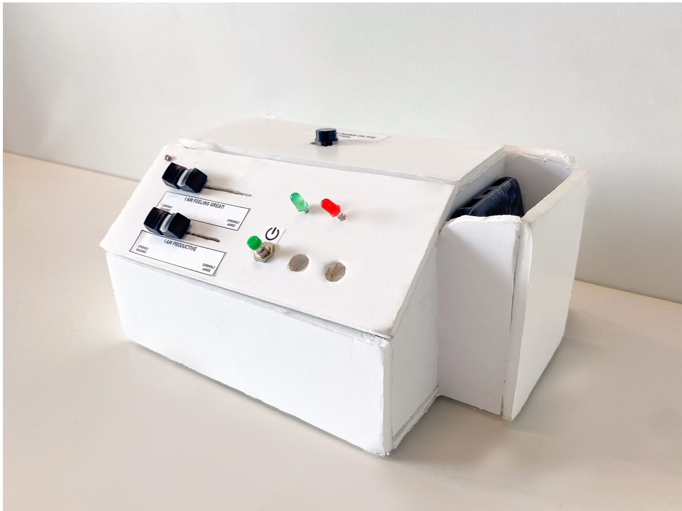
Figure 1: The first contextual iteration probe. Users can at any time input their (dis)agreement the the statements "I am feeling great" and "I am being productive". A sensor to detect phone usage, an LDR, and a temperature sensor were also included.
